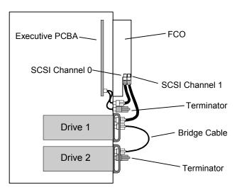
Figure 6-6 TLS-62xx and 82xx Cabling Diagram
